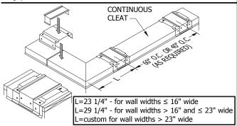
STEP 2: Installing Anchor Clips at Corners & Along the Parapet Locate anchor clips as shown. Pull clips snugly against the outside face. Place four (4) screw fasteners in the top of the clip. Place two (2) SS ring shank nails in the clip face (outer holes). Position the joint splice over the center of the clip and install as shown using two (2) SS ring shank nails thru aligning holes. Joint splices should be installed at ALL clip locations.
