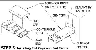
Install end caps and end terms by hooking face and snapping back into place. End caps must be restrained from moving by securing the end cap to the clip using a stainless steel screw or rivet (by installer) through the roof side leg of the end cap. End terms should be restrained similarly if no fasteners are previously installed in the end term wall flange.
