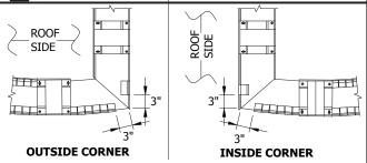
**STEP 2: Installing Cont. Cleats & Corner Supports At Corners** Continuous cleats are to be placed at all corners to support the cap. Secure clips using fasteners provided. Field cut each cleat to fit aproximately 3" from corner.
